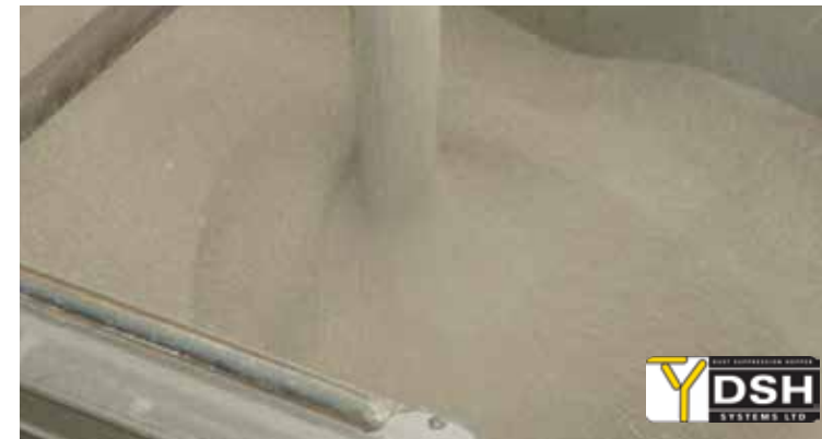
With DSH systems, there is no dust generation on impact. Radial flow occurs away from the impact point.
